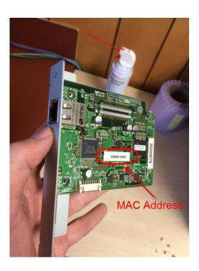
To see if you already have a LAN installed, check on the back of the printer. If you are able to see an Ethernet Cable receiver, you have a LAN Card installed.
