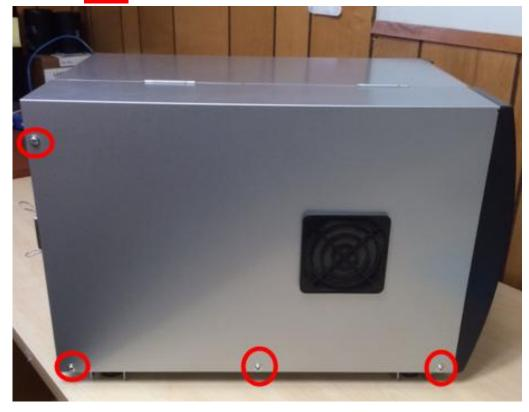
Lift Cover and remove screws from both Hinges and the remaining screws from the Side Cover
